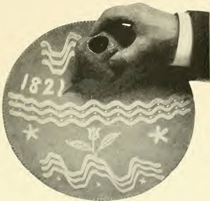
9. SINGLE QUILL SLIP CUP. For Ornamental Slip-Tracing.
